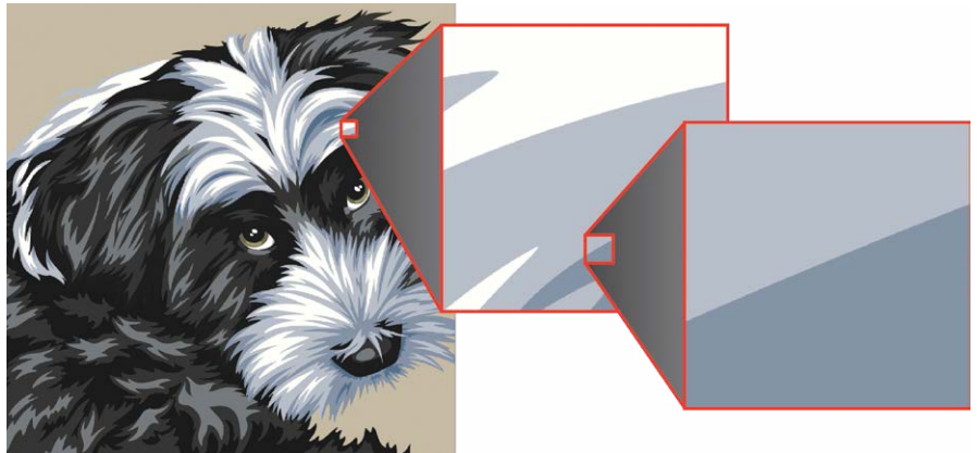
Vector images are based on mathematical equations and do not contain pixels. When zooming in for a closer look, Yoda's vector lines stay crisp and sharp.
