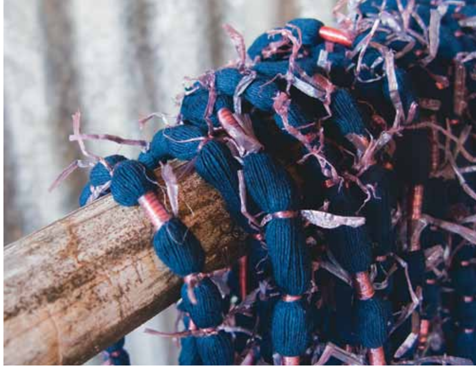
Mudmee tying process; threads after dyeing
